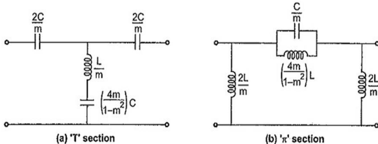
Fig 25 m-Derived high pass filter
