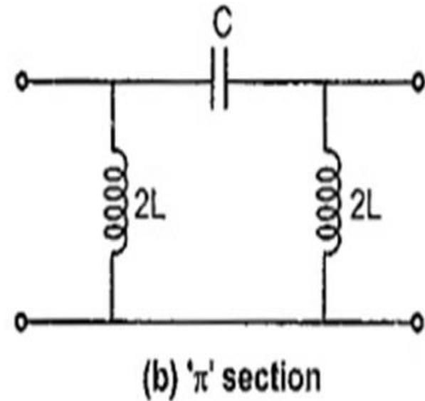
Fig 6 Prototype T and  $\pi$  high pass filter
