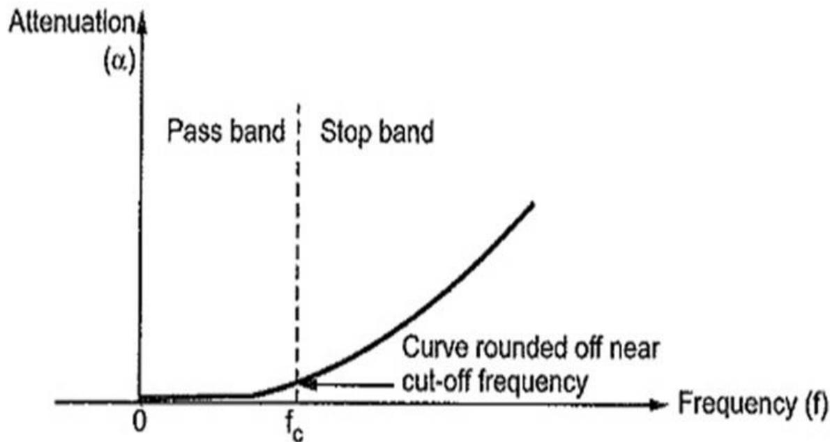
Fig 18 Attenuation constant with frequency
