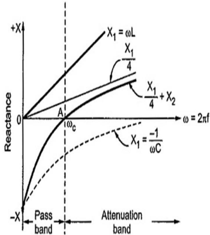
Fig 2 Reactance Frequency sketch for prototype low pass filter
