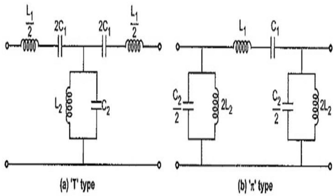
Fig 12 Prototype T and  $\pi$  band pass filter
