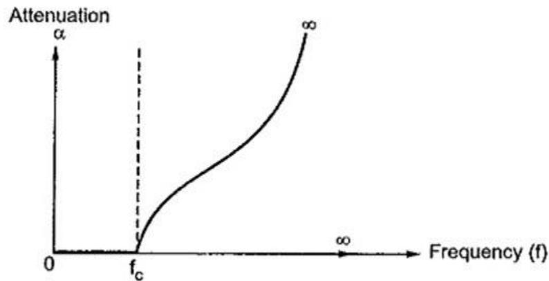
Fig 4 Variations of attenuation constant with frequency
