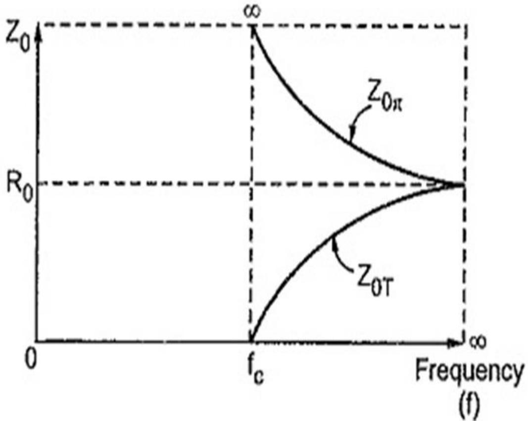
Fig 8 Variation of Characteristics impedance with frequency
