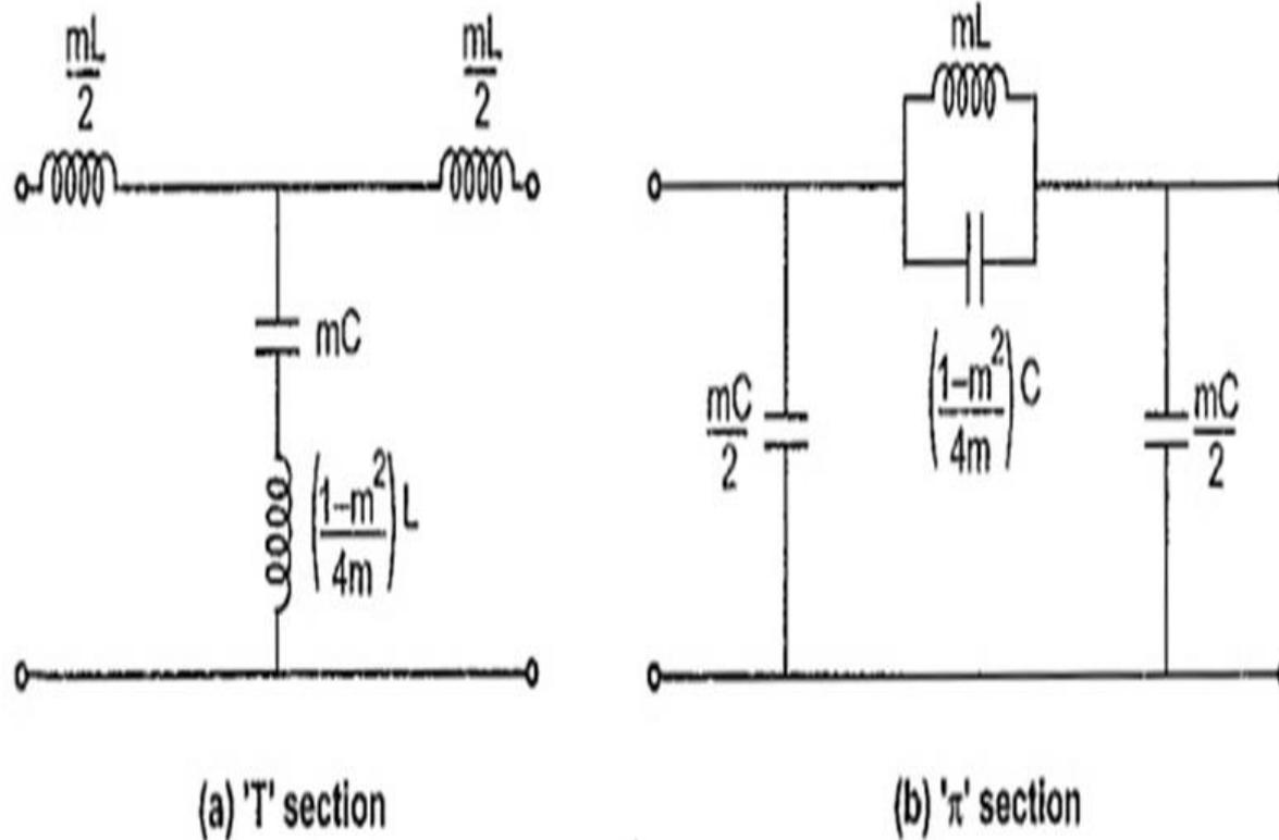
Fig 23 m-Derived Low Pass Filter
