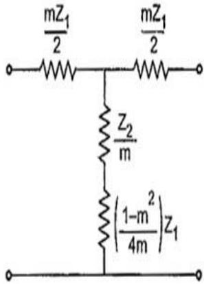
**Fig 20 m-Derived T section**
