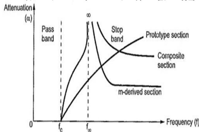
Fig. 27 Variation of attenuation constant in prototype, m-derived, and composite section
