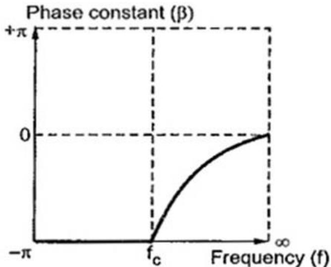
Fig 10 Variations of phase constant with frequency
