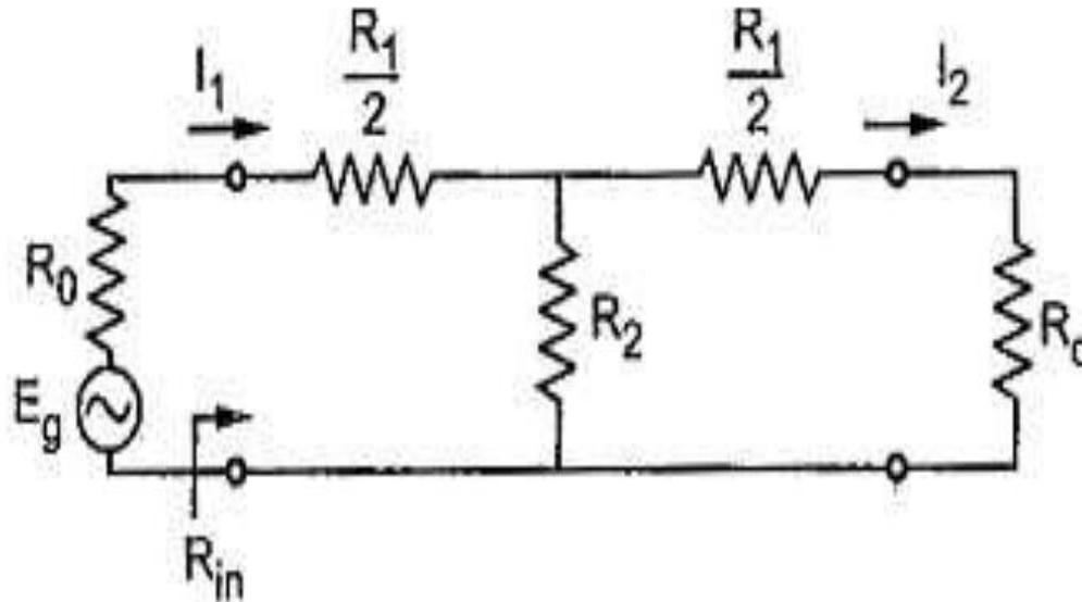
Fig. 1 Symmetrical T Type Attenuator
