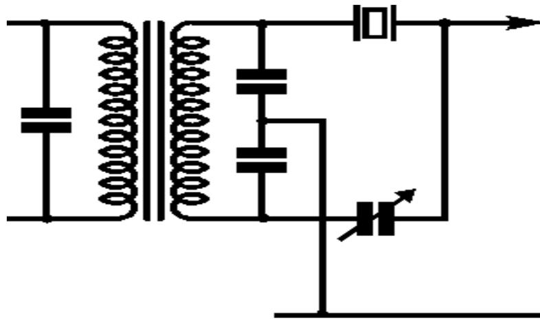
Diagram of filter using a single quartz crystal
