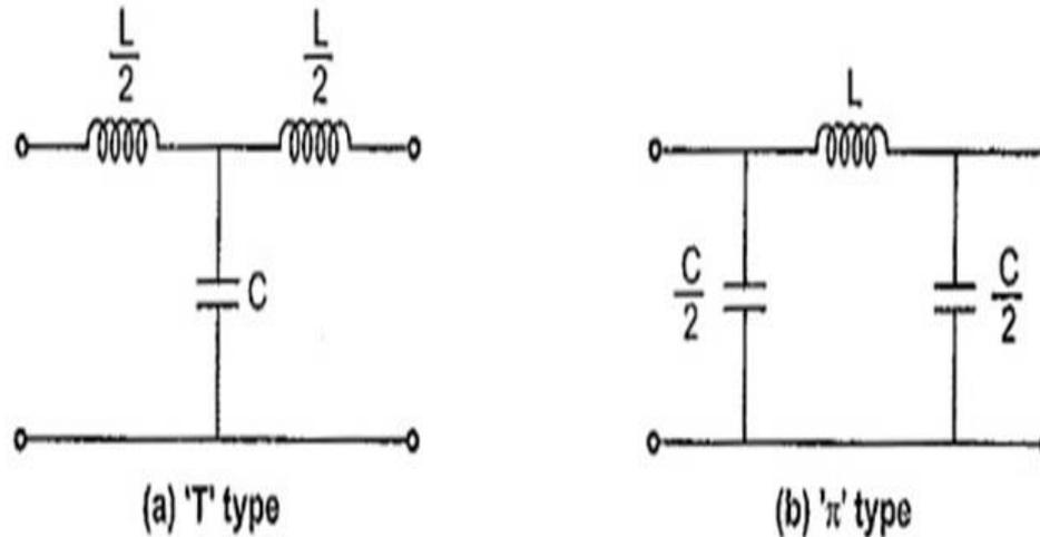
Fig 1 Prototype T and  $\pi$  low pass filter
