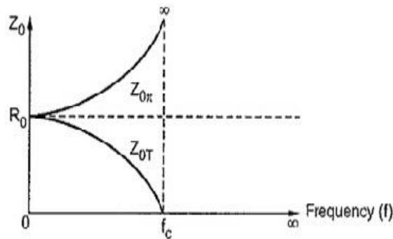
Fig 3 Variation of characteristics impedance with frequency
