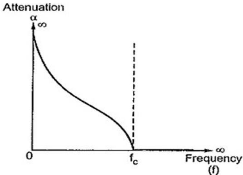
Fig 9 Variation of attenuation constant with frequency
