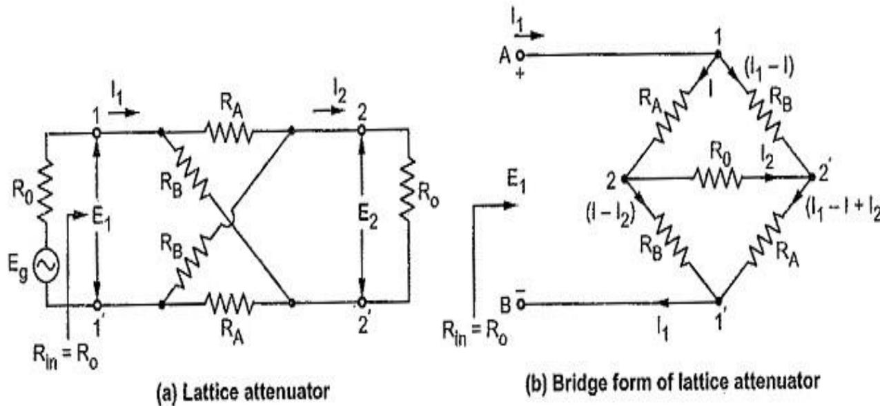
Fig. 3 Symmetrical Lattice Type Attenuator
