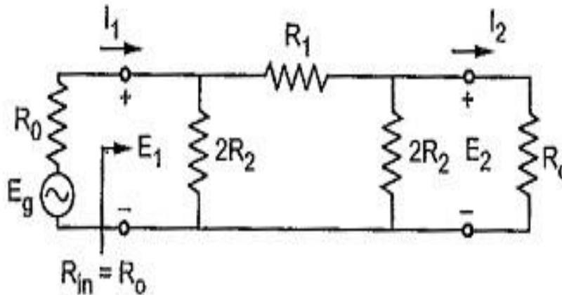
Fig - 2 **Symmetrical  $\pi$  Type Attenuator**
