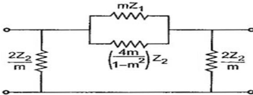
Fig 22  $m$ -Derived  $\pi$  section
