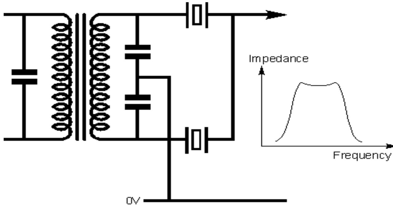
Diagram of half lattice crystal filter
