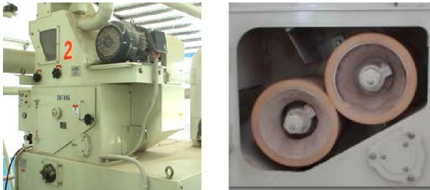
Fig. 17. Dehusking principle of rubber roll huller.
