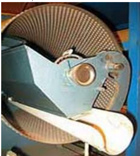
Working principle of the indented cylinder separator
