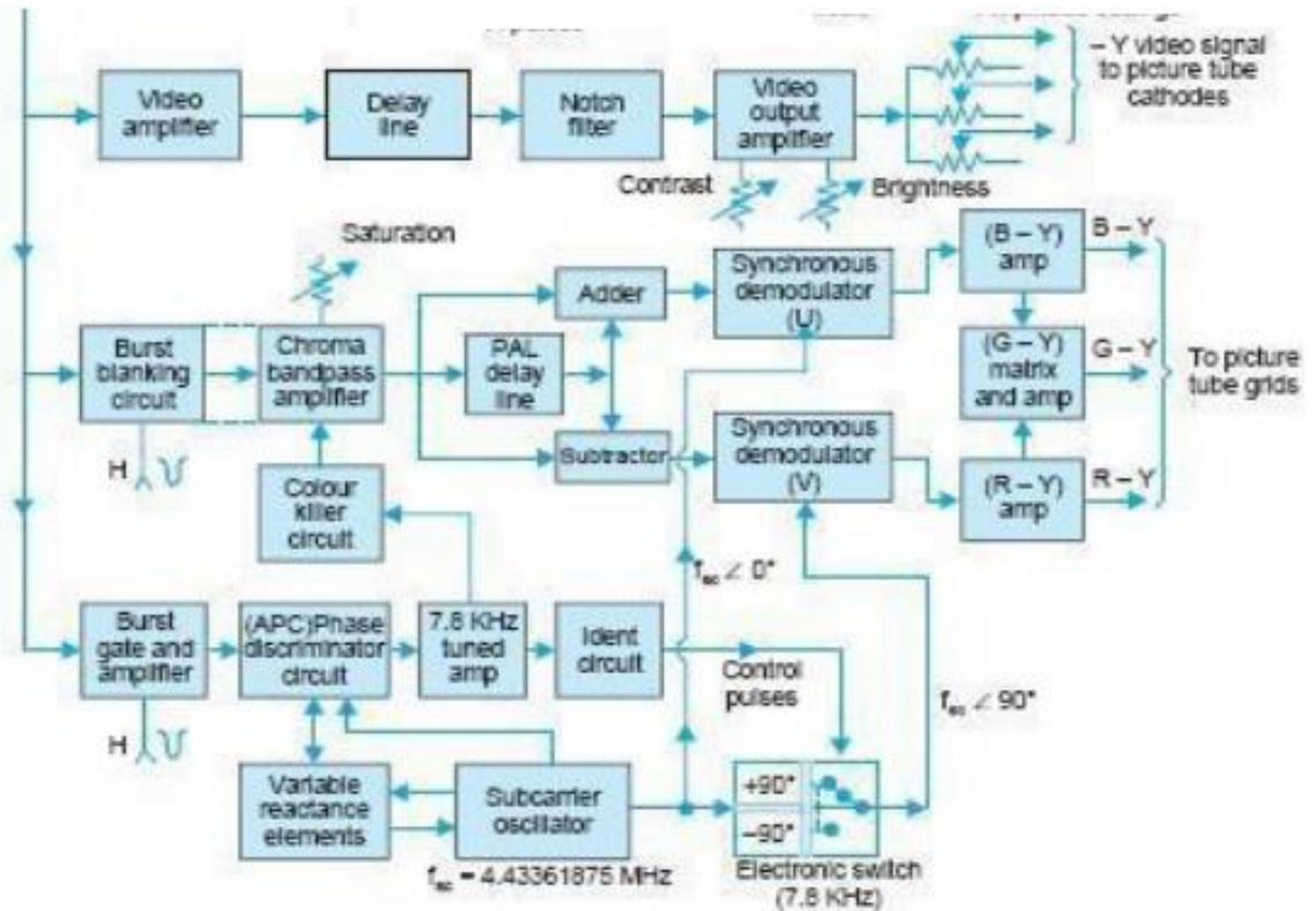
**Figure. Block diagram of a PAL-D colour receiver.**
