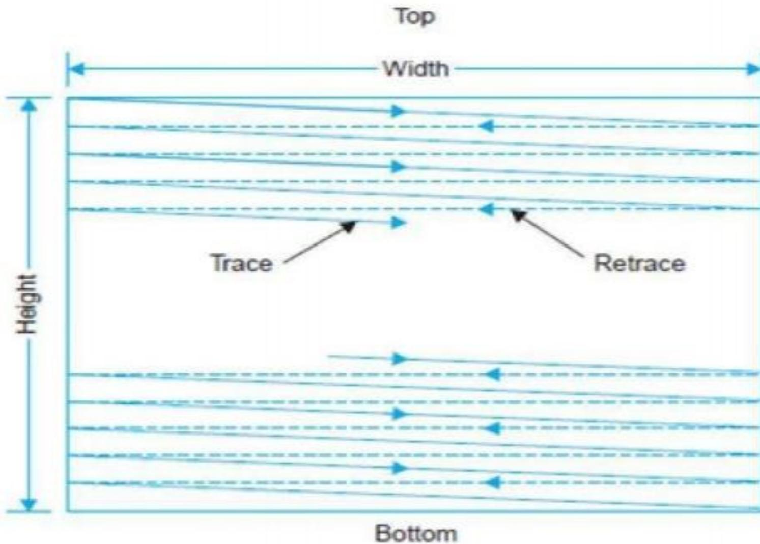
**Figure. Path of scanning beam in covering picture area**
