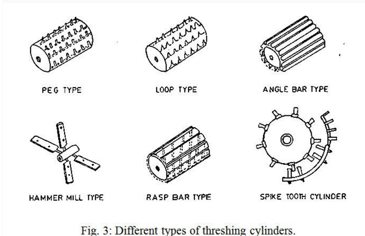
**Fig. 3: Different types of threshing cylinders.**
