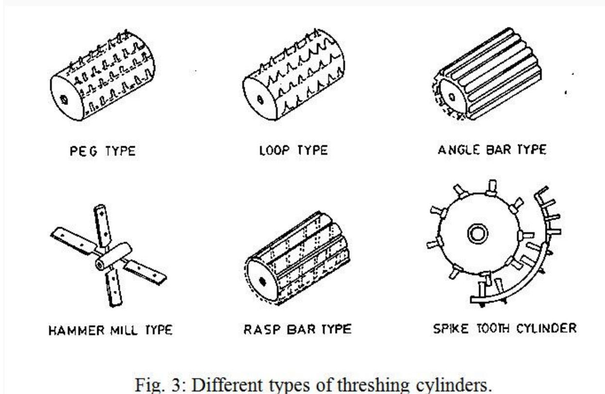
**Fig. 3: Different types of threshing cylinders.**
