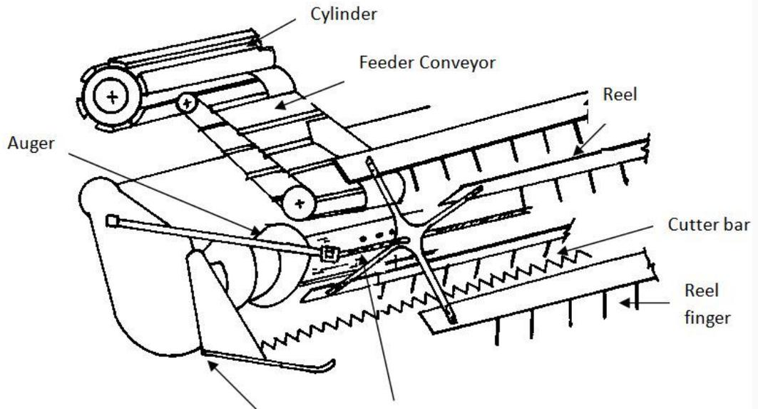
Fig. 5: Cutter bar assembly of a combine harvester.
