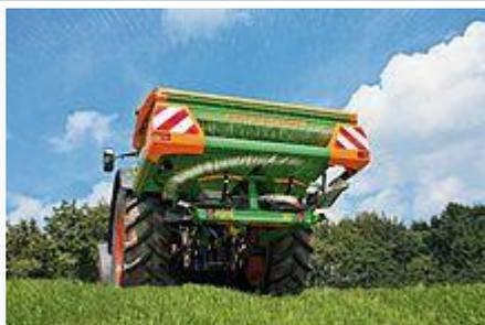
View of a tractor-operated broadcast seeder moved by [three-point hitch](#) and driven by [PTO](#) shaft
