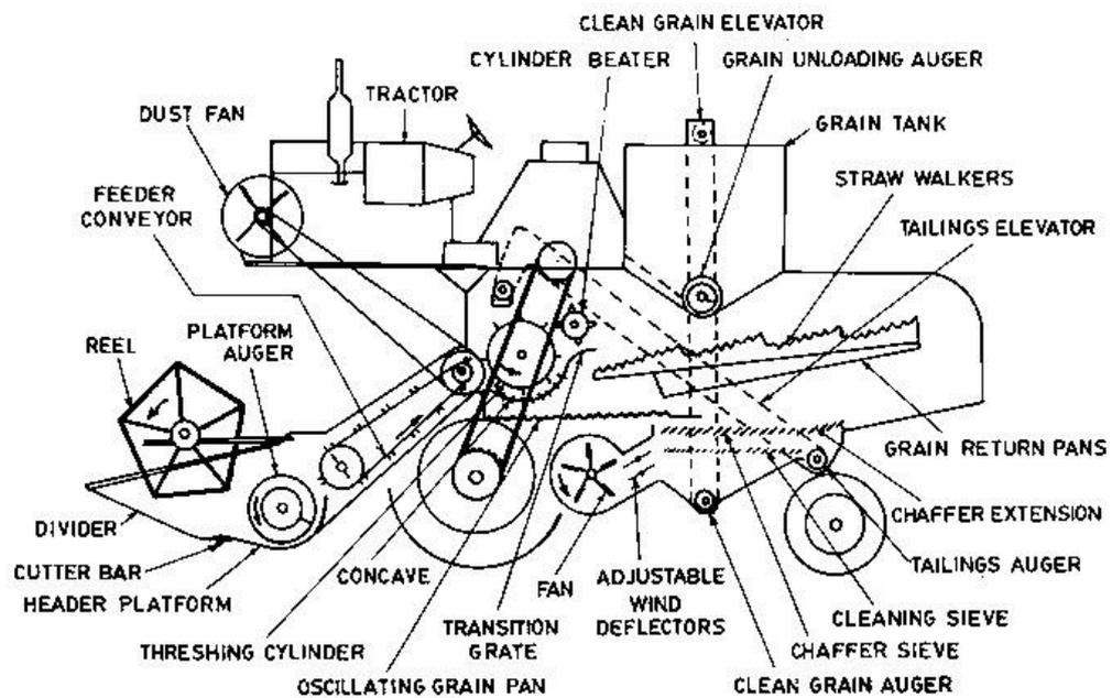
Fig. 4: Details of a tractor operated combine harvester.
