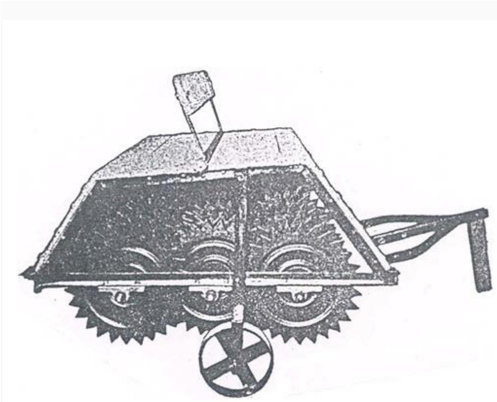
Fig. 6: Olpad thresher
