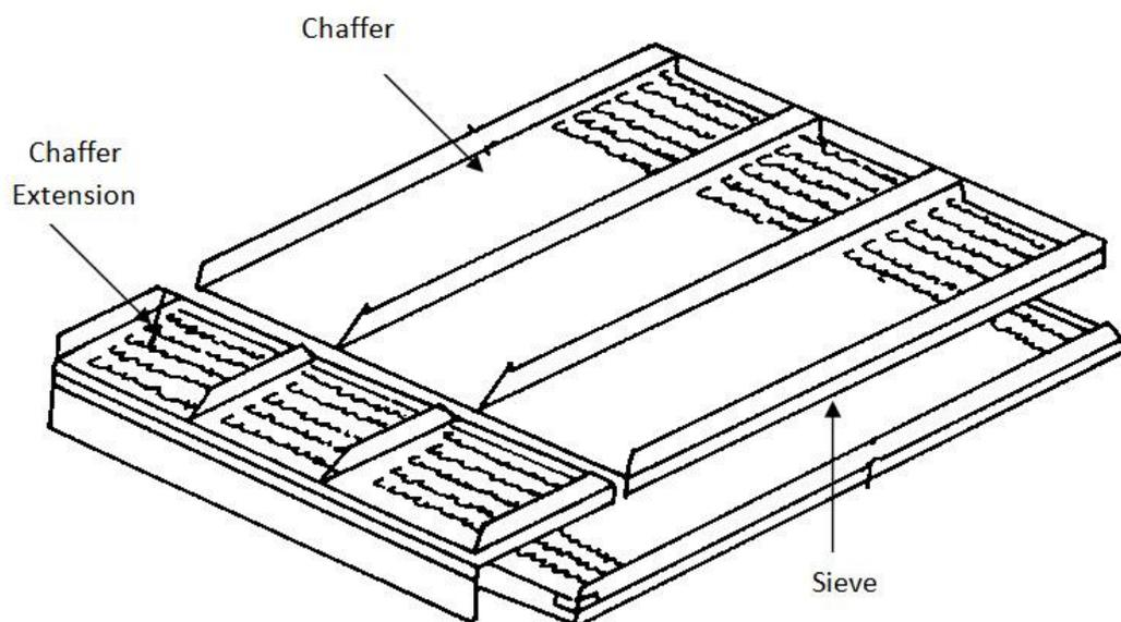
Fig. 7: Cleaning unit of a combine harvester.
