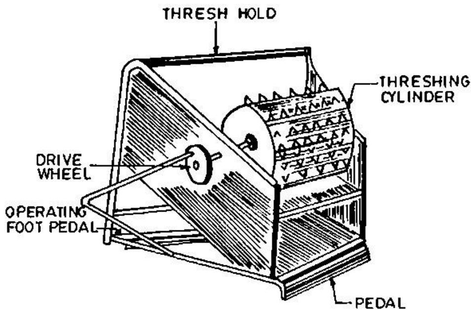
Fig. 7: Pedal operated paddy thresher.
