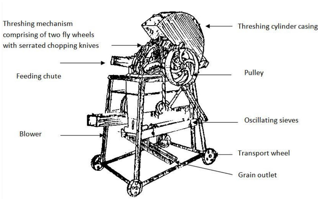
Fig. 4: Detail components of chaff cutter type thresher.
