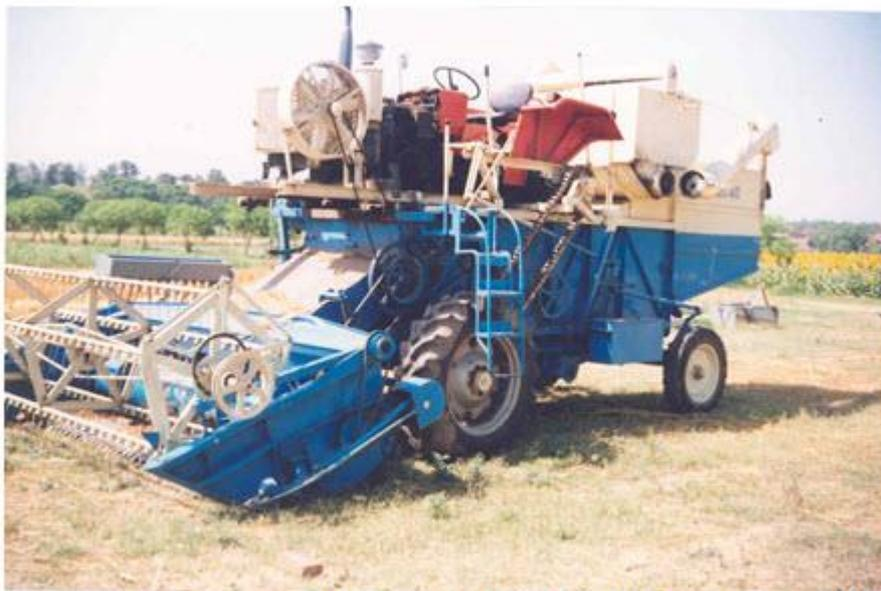
Fig. 2: A grain combine with 55-hp tractor mounted on it.
