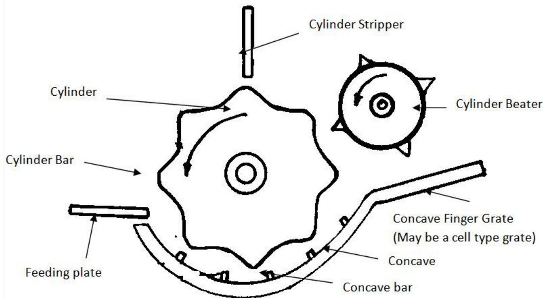
Fig. 6: Threshing unit of a combine harvester.
