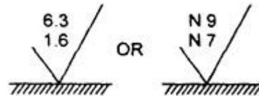
**Fig. 1.10** Invocation of the maximum and minimum limits of surface roughness.
