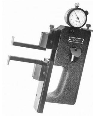
Groove Gages are mechanical metrology instruments used in inspection applications to confirm dimensions of machined internal features such as ring grooves, undercuts, inside diameters, etc. They are generally configured to fit through the confines of narrow bores and then be opened to take the measure of any internal features. Some are used to measure concentricity.
