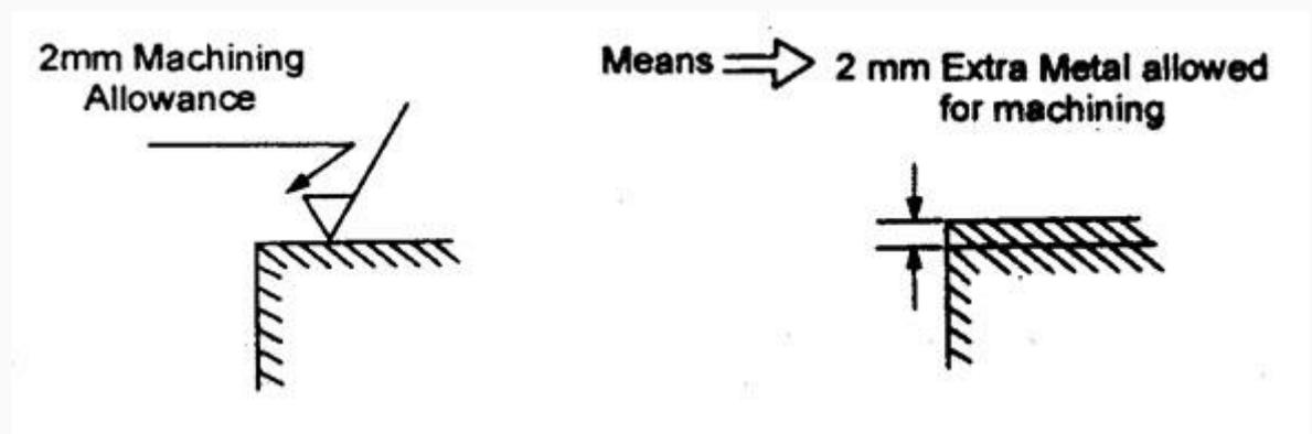
**Fig. 1.6 Indication of machining allowances**
