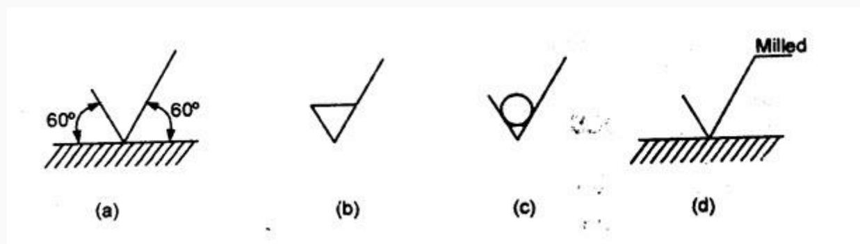
**Fig. 5.8 Symbols used for indication of surface roughness**
