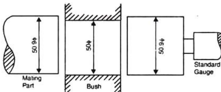
**Fig 1.39. Use of a Standard Gauge.**
