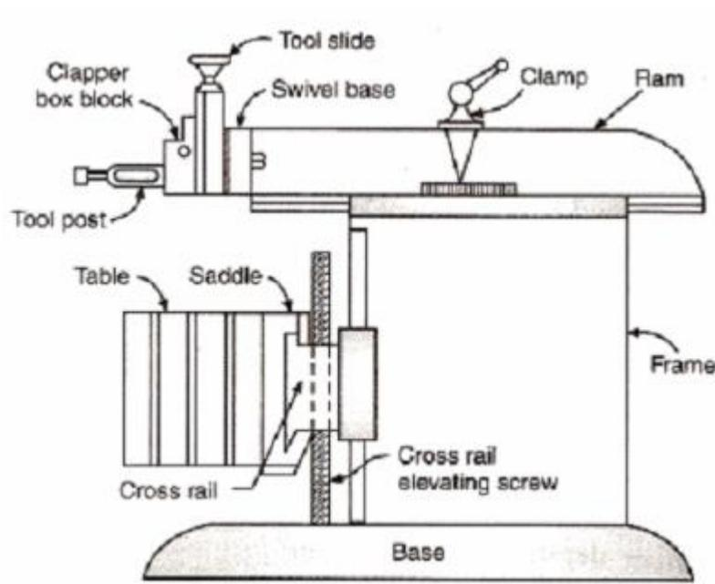
**Construction:** The main parts of the Shaper machine is Base, Body (Pillar, Frame, Column), Cross rail, Ram and tool head (Tool Post, Tool Slide, Clamper Box Block).
