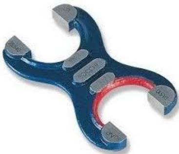
Snap gauges are simple mechanical inspection instruments used to verify that the outside dimensions of parts are within their specified tolerances. Key specifications include features, range, and accuracy. Snap gauges can be either fixed or adjustable devices. Fixed snap gauges are manufactured to set measurements whereas adjustable snap gauges can be set to measure over ranges of measurements.
