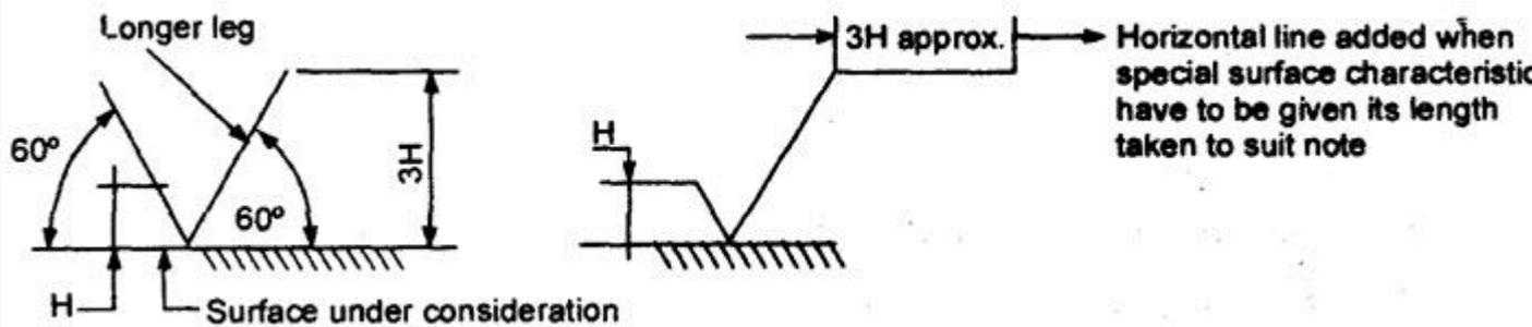
**Fig. 1.7 Basic symbol for indication of surface roughness**
